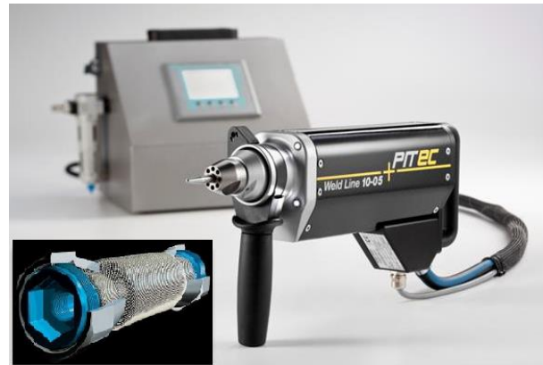
Figure 1. The PIT hand held device and controller with the fluidic muscle from Festo (far left).
