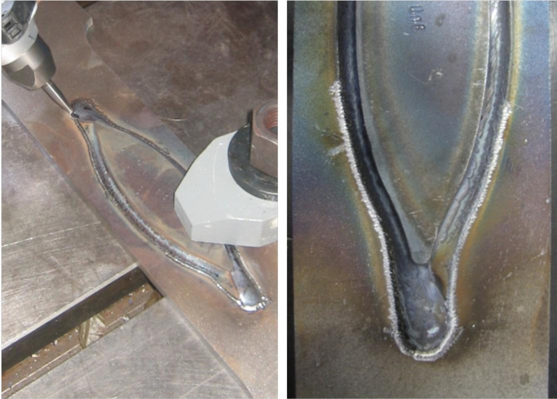
Figure 4: HFMI-treatment at weld toe of end-of-seam specimens
