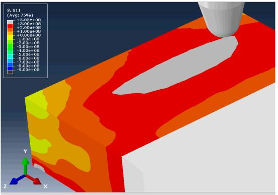
Half symmetrical model of the weld specimen – loaded with  $\sigma_{xx-load}$ =200MPa
