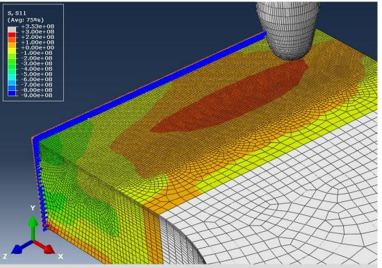
Half symmetrical model of the weld specimen
