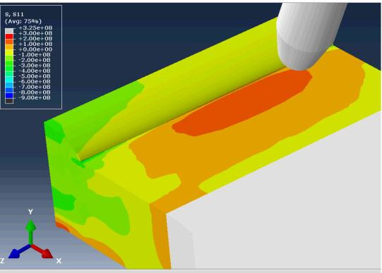
Half symmetrical model of the weld specimen – one load cycle after HFMI ( $\sigma_{xx-load} \le \pm 450 MPa$ )
