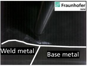
During this process, a hardened cylindrical metal pin with a spherical tip impacts the weld toe surface with high frequency and induces local plastic deformation.
