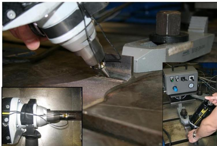
**Fig. 5: Strain gauge measurement at hardened pin [6]**
